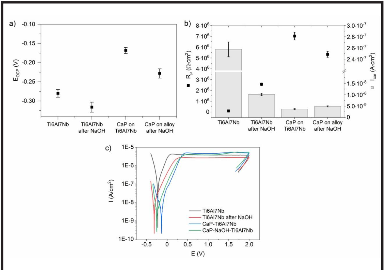
FIG. 6. Corrosion characteristics of Ti6Al7Nb alloy without and with CaP coatings in PBS solution: a) open circuit potential  $E_{\text{OCP}}$ , b) polarization resistance  $R_p$  and corrosion current density  $I_{\text{cor}}$ , c) potentiodynamic polarization curves.
