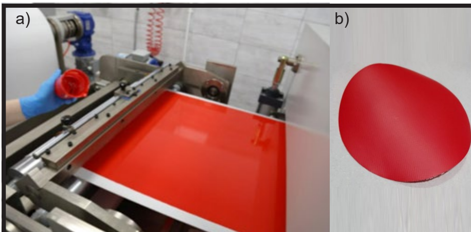
FIG. 4. The fabric coating process (a) and a cutout of the resulting coated fabric sample (b).
