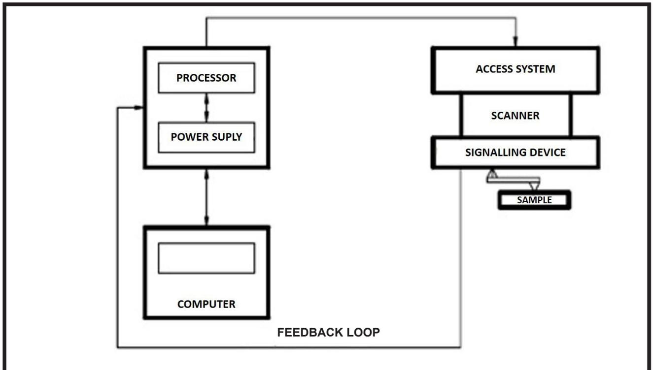
FIG. 4. Block diagram of the atomic force microscope [6].
