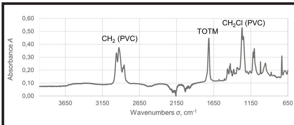
FIG. 11. FTIR-ATR absorption spectrum of the transparent drain.
