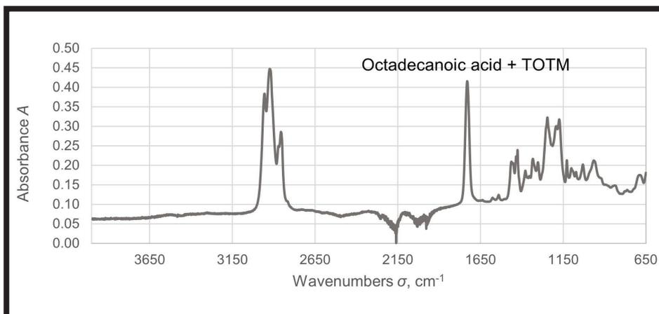
FIG. 10. FTIR-ATR absorption spectrum of the amber drain.
