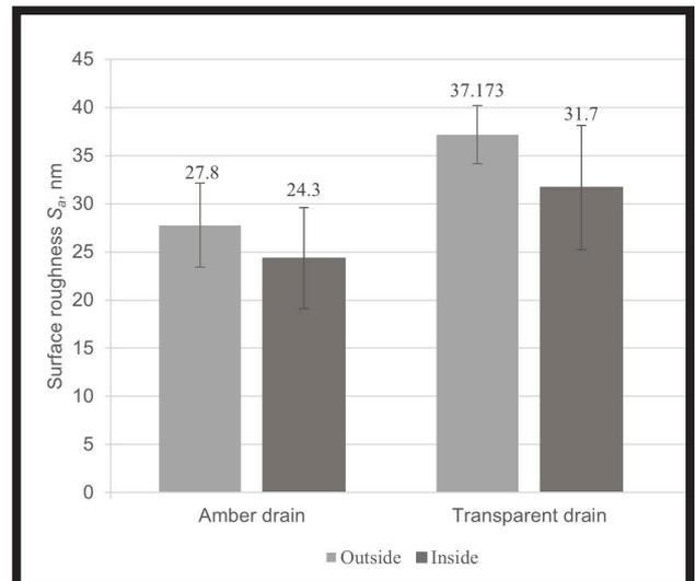
**FIG. 14. The average values of the surface roughness ( $S_a$ ) depending on the type of the drain and side of the tested surface.**
