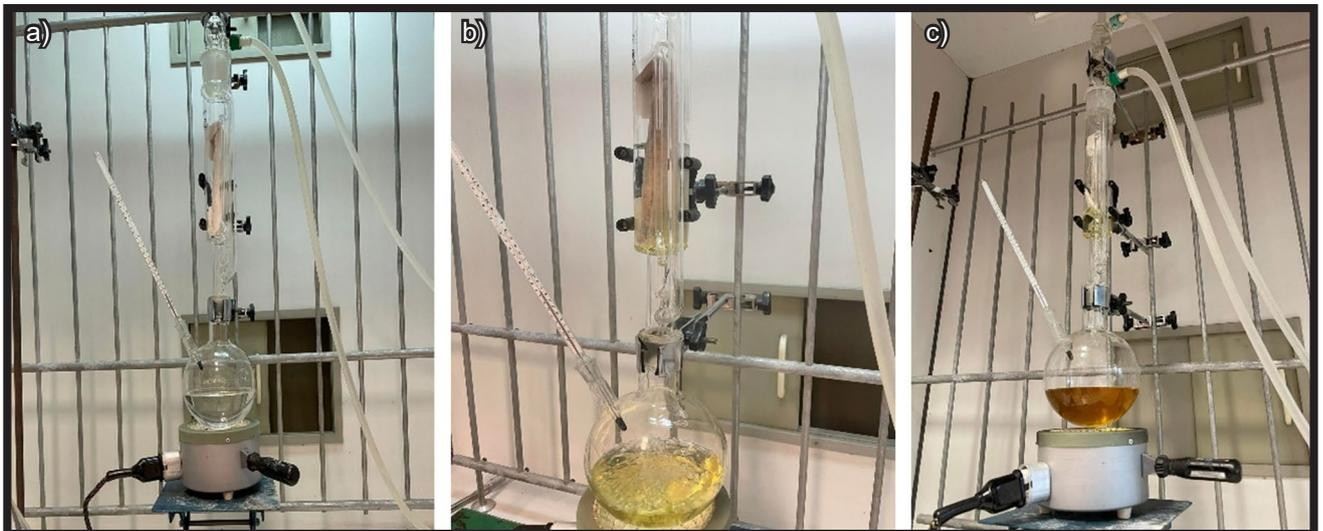
FIG. 4. Process of extracting betulin from birch bark: a) before heating, b) during boiling, c) high concentration of botulin.
