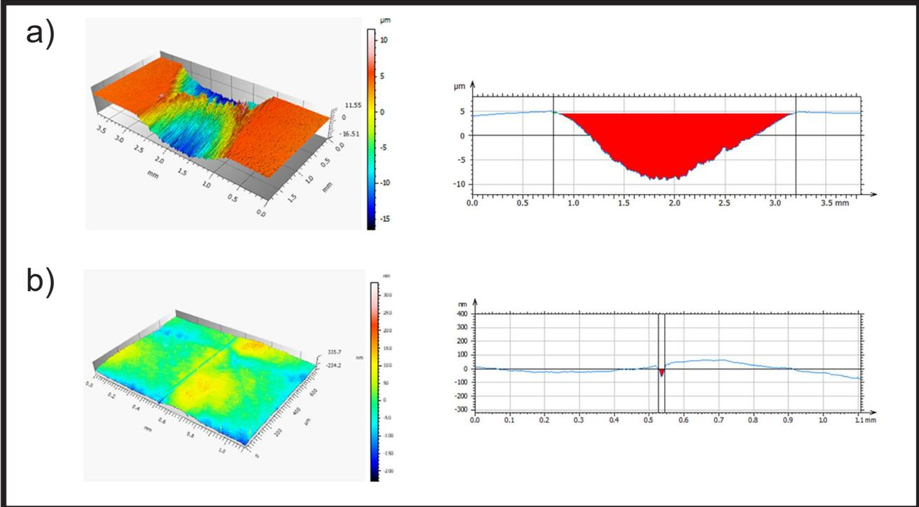
FIG. 6. The axonometric image of the trace of wear and the wear profile in a cross-section during technical dry friction: a) Ti13Nb13Zr, b) Ti13Nb13Zr DLC.
