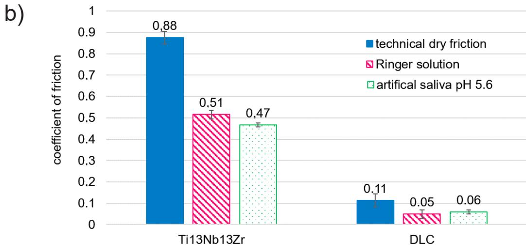
FIG. 5. a) Sample plots of the coefficient of friction, b) mean coefficient of friction.
