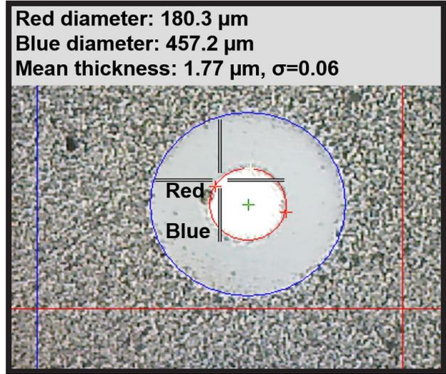
FIG. 2. An image recorded during thickness measurement of the DLC coating.
