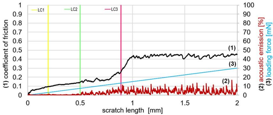
FIG. 4. Scratch test results - graph of variation of loading force (Fn), coefficient of friction ( $\mu$ ), acoustic emission.
