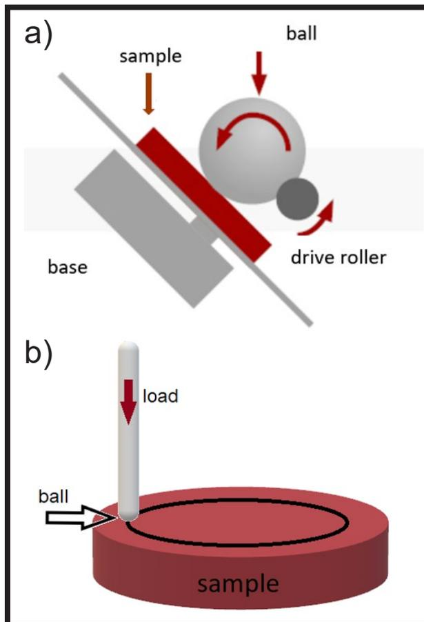
FIG. 1. Friction pair in Calotest (a), friction pair in TRB<sup>3</sup> (b).
