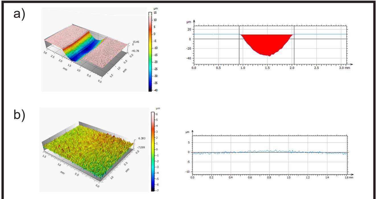
FIG. 8. The axonometric image of the trace of wear and the wear profile in a cross-section during friction in an artificial saliva environment: a) Ti13Nb13Zr, b) Ti13Nb13Zr DLC.
