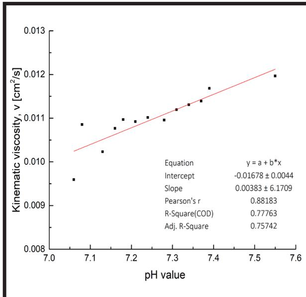
FIG. 3. The correlation between the kinematic viscosity ( $v$ ) and pH value of examined solutions.
