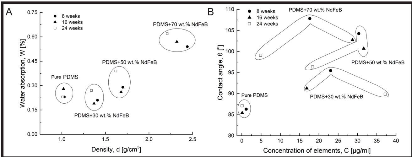
**FIG. 5. The correlation between chosen parameters. (A) The water absorption (W) vs density (d) for the examined materials. (B) The contact angle of surface of materials ( $\theta$ ) vs the concentration of elements in solution (C).**
