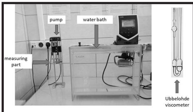
**FIG. 1. iVisc system for kinematic viscosity determination.**
