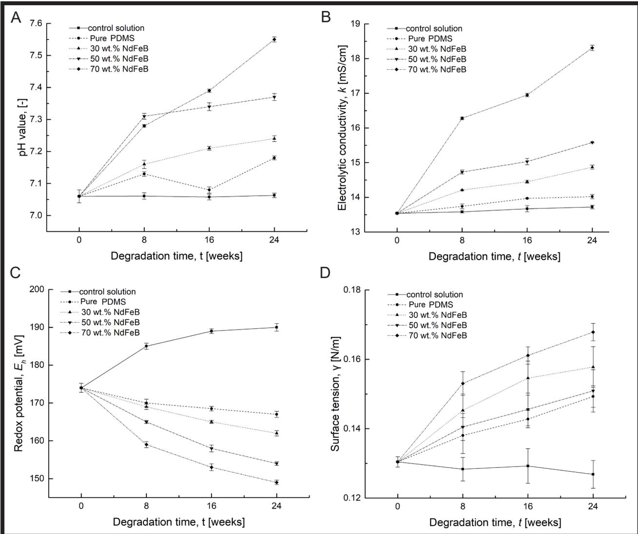
**FIG. 2. Results of physiochemical properties of solutions vs incubation time: (A) pH value; (B) Electrolytic conductivity; (C) Redox potential; (D) Surface tension.**
