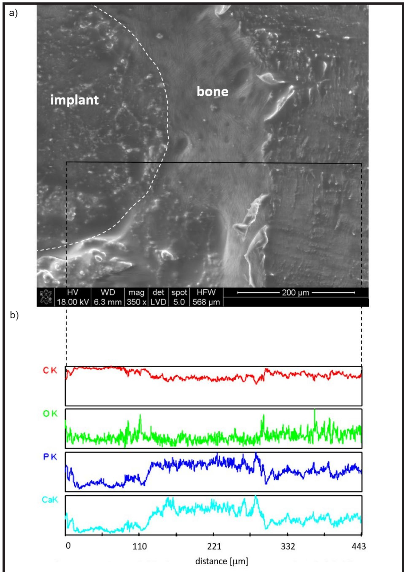
FIG. 4. a) SEM image of bone-implant section; b) EDS analysis of element composition (carbon, oxygen, phosphorus, calcium) along the line marked on the SEM image.
