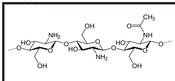
FIG. 1. Structure of a chitosan molecule.
