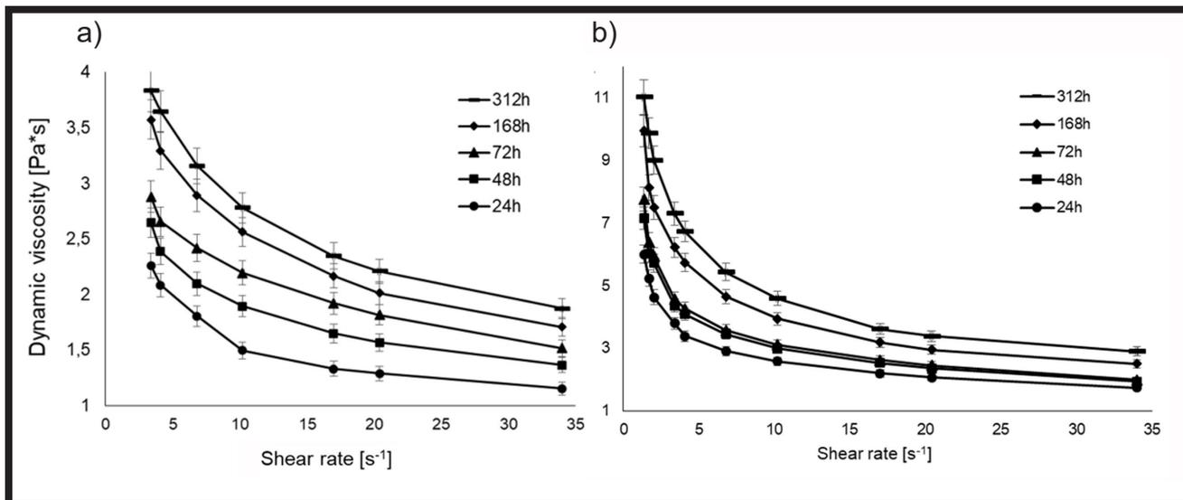
FIG. 4. Comparison of dynamic viscosity of chitosan gel with lactobionic acid (a) and mandelic acid (b) depending on the time.
