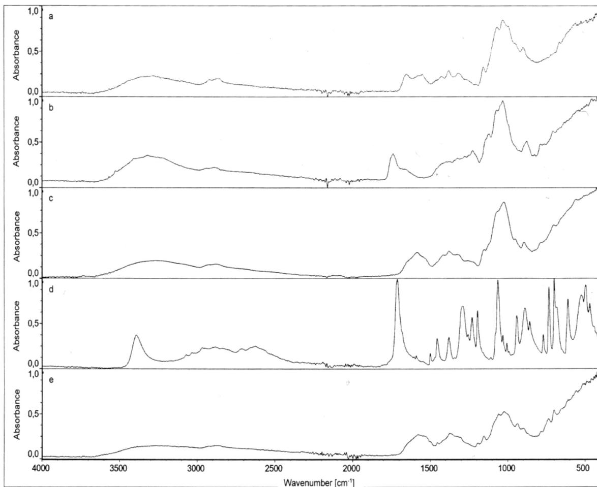
FIG. 5. FTIR spectra of chitosan (a), lactobionic acid (b), mandelic acid (d) and chitosan hydrogels with lactobionic acid (c) and mandelic acid (e).
