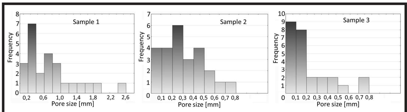
FIG. 3. Frequency of the pore size in a particular range for samples 1, 2 and 3.
