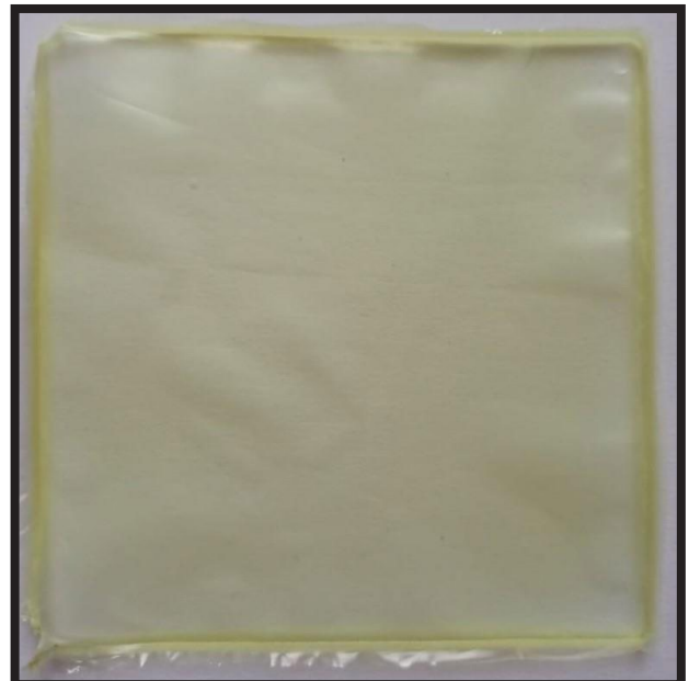
FIG. 2. Image of the film made from the mixture of 1.5% low molecular weight HA with egg albumin.
