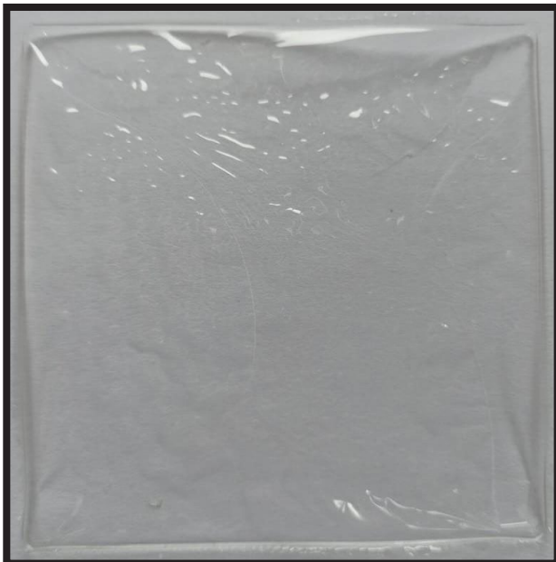
FIG. 1. Image of the film made from the 1.5% low molecular weight HA solution.
