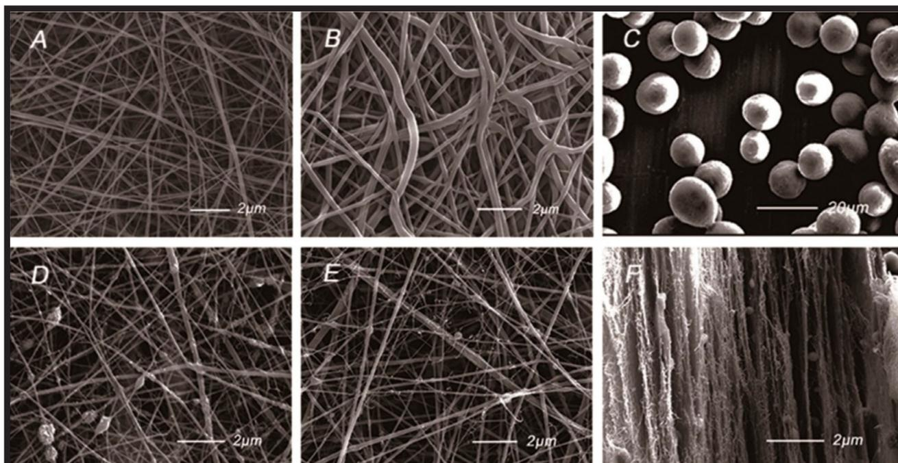
FIG. 4. SEM images of the microstructure of the Gln/CS composite membrane before (A) and after (B) crosslinking; (C) Electrospun AMP@PLGA; The layer of Gln/CS/nHAp by magnetic stirring (D) and ultrasonic dispersion (E); (F) Cross-sectional image of the membrane [40].
