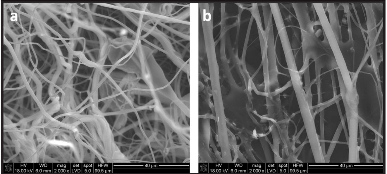
**FIG. 3. Unmodified cellulose acetate (CA) fibers (a) and CA fibers surface modified by EPD method in  $\text{SiO}_2$  suspension (b) [35].**
