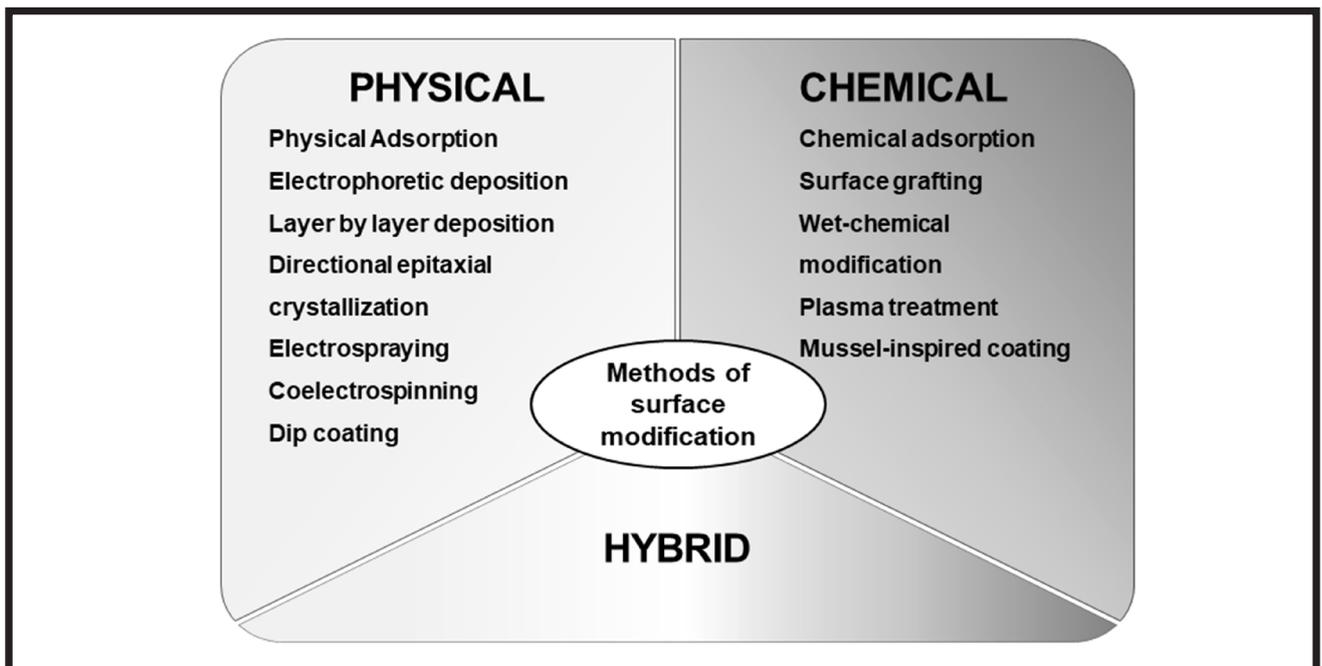
FIG. 1. Methods of fibers surface modification.
