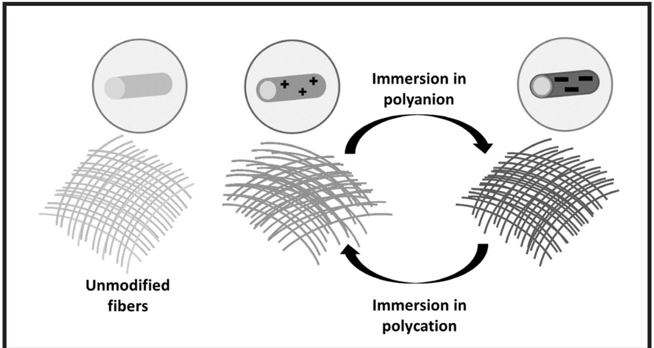
FIG. 6. Schema of the LBL process.
