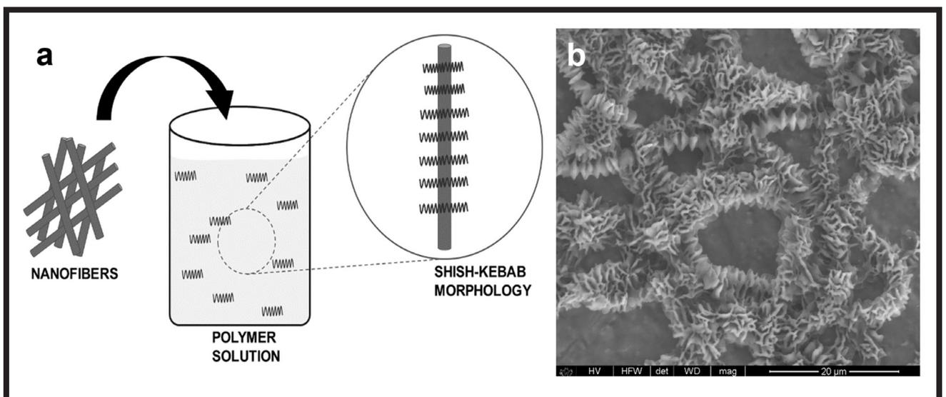
FIG. 7. Schema of the directional epitaxial crystallization process (a) and SEM image of shish-kebab morphology (b) [55].
