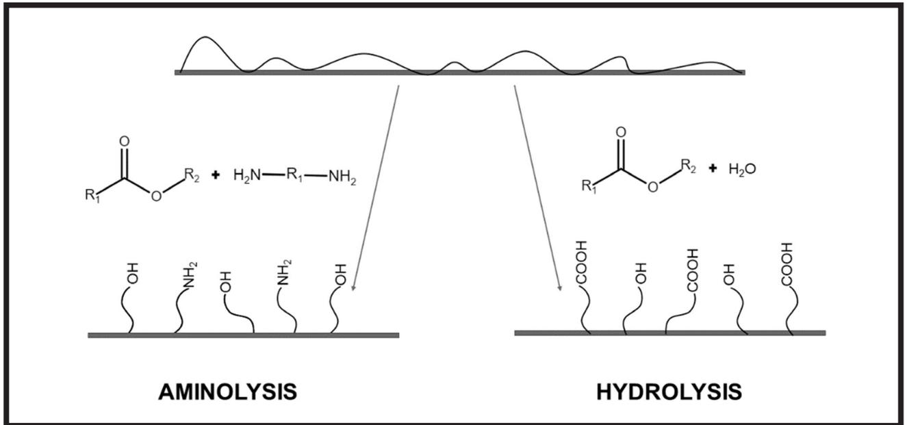
FIG. 8. Surface chemistry after hydrolysis and aminolysis.
