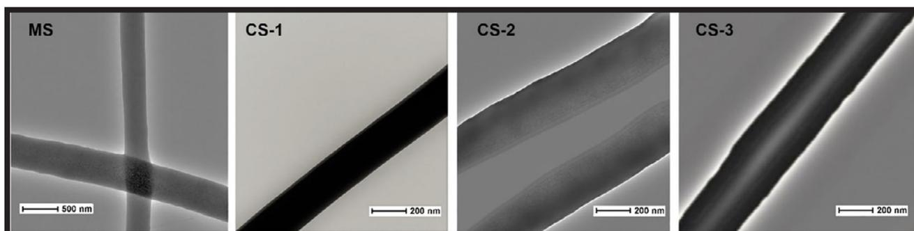
FIG. 5. TEM images of monostructural and core-shell fibers [45].
