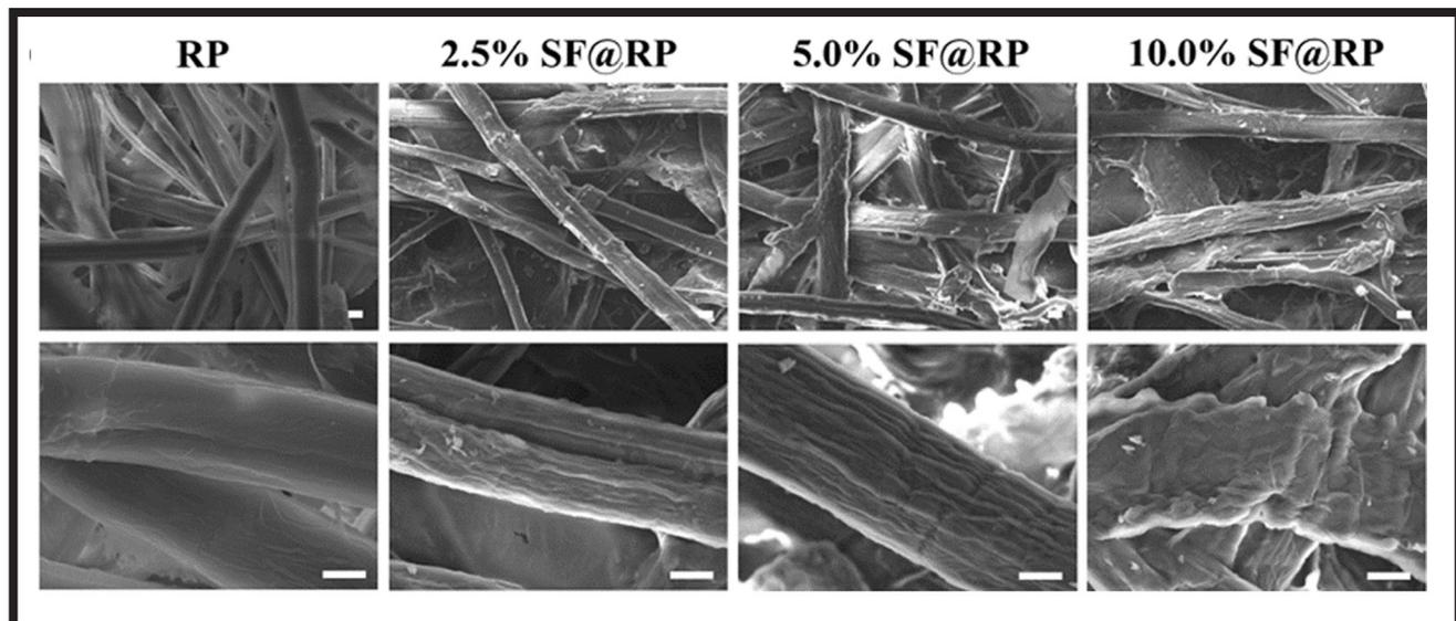
FIG. 2. FESEM pictures of rice paper (RP) and SF@RP (silk fibroin@rice paper) at different concentrations of SF [29].
