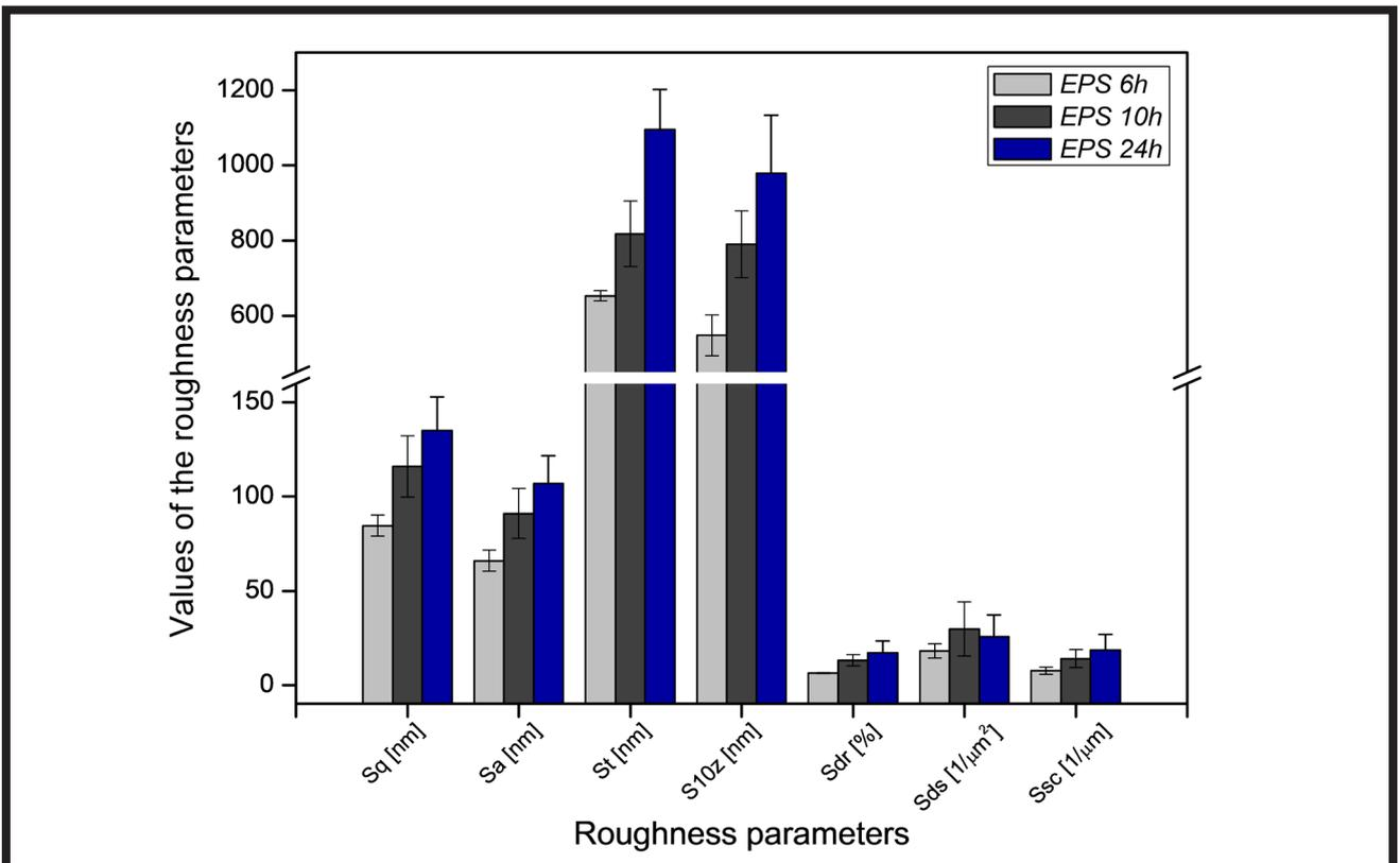
FIG. 2. Values of selected roughness parameters for EPS samples.
