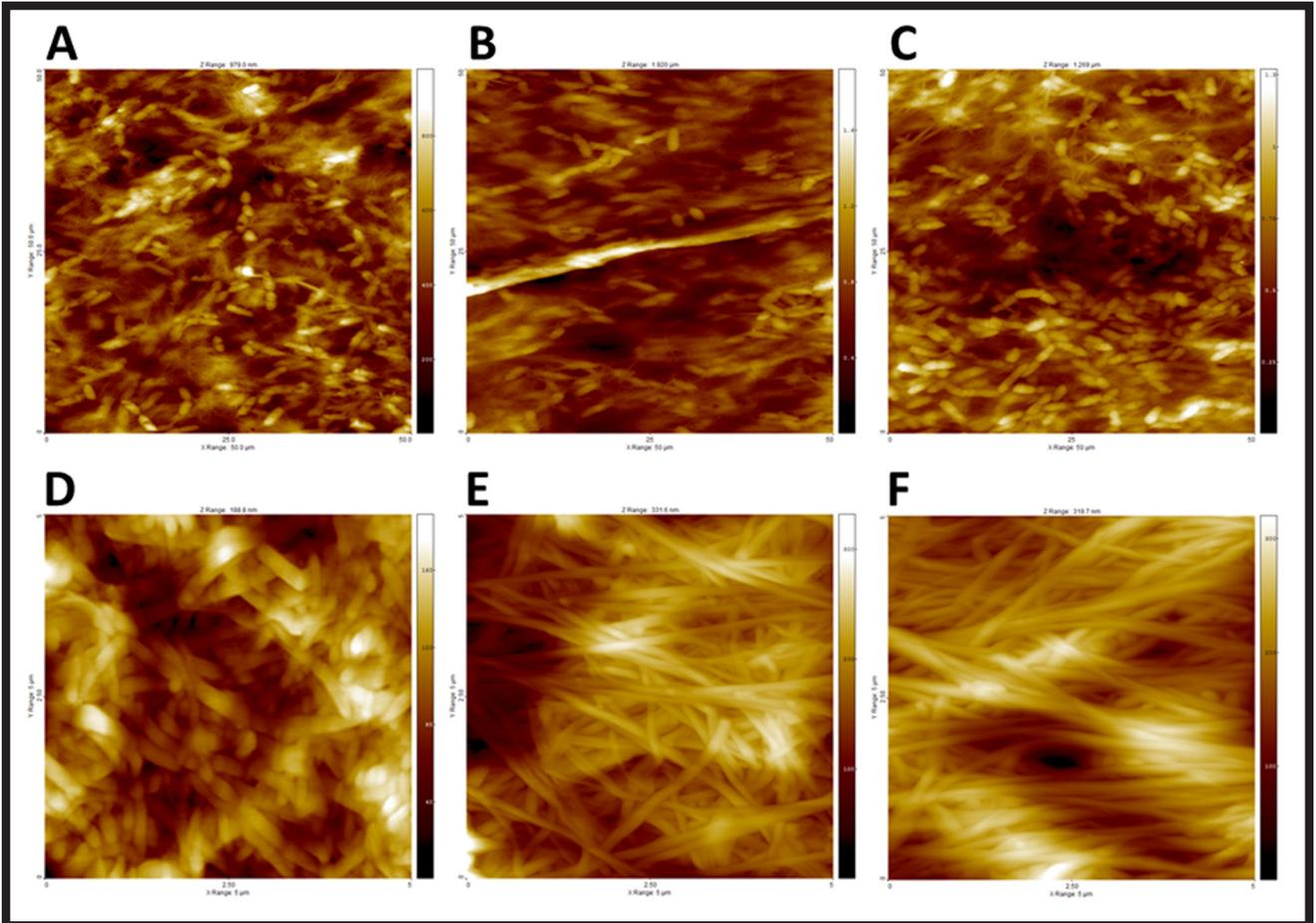
FIG. 1. AFM images of EPS surface for selected growing time periods, scan sizes 50 μm x 50 μm (A-C) and 5 μm x 5 μm (D-F).
