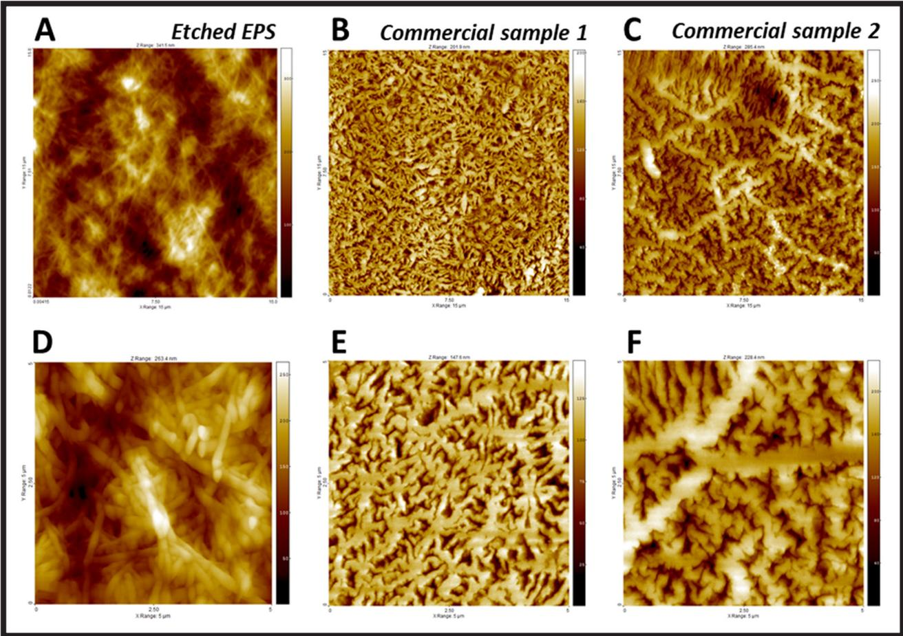
FIG. 3. AFM images of etched EPS surface and reference samples, scan sizes 15 μm x 15 μm (A-C) and 5 μm x 5 μm (D-F).
