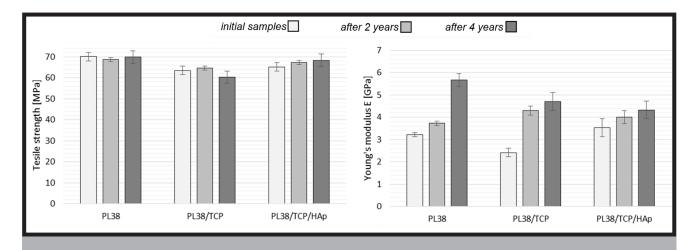
FIG. 5. Comparison of average  $R_m$  and E values obtained during mechanical testing of dumbbell-shaped specimens of the initial samples, after 2 and after 4 years.
