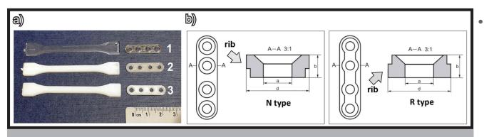
FIG. 1. a) Examples of dumbbell-shaped specimens and fixation miniplates used for testing. 1 - PL38; 2 - PL38/TCP; 3 - PL38/TCP/HAp; b) Schematic sketches of the I-shaped four-hole miniplate: type "N" with reinforcing rib from the bottom; type "R" with reinforcing rib from the top.
