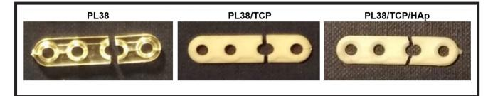
FIG. 10. Examples of miniplates after the mechanical testing. The characteristic manner of fracture can be seen.
