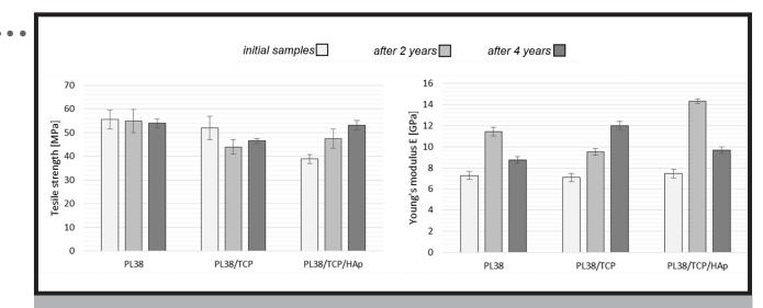
FIG. 8. Comparison of mechanical test results ( $R_m$  and E) of the "N" type fixation miniplates of the initial samples, after 2 and after 4 years.
