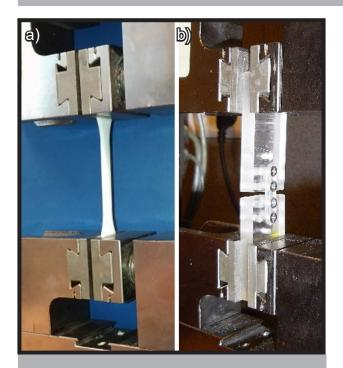
FIG. 2. a) Dumbbell-shaped specimen mounted and ready for testing; b) Simulated model of osteosynthesis with fixation miniplate.
