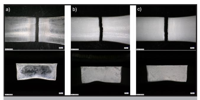
FIG. 4. Example of microscopic images of sample fracture (KEYENCE VHX-500, mag. x30; x50): a) PL38; b) PL38/TCP; c) PL38/TCP/HAp.
