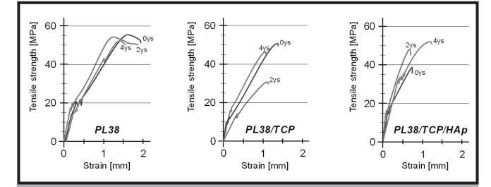
FIG. 6. Example tensile curves of "N" type miniplates. 0ys - initial samples; 2ys - tested after two years; 4ys - tested after four years.
