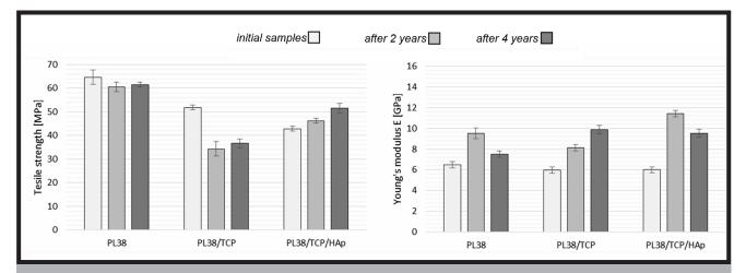
FIG. 9. Comparison of mechanical test results ( $R_m$  and E) of the "R" type fixation miniplates of the initial samples, after 2 and after 4 years.
