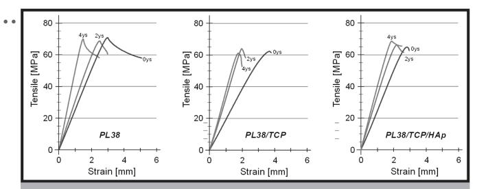
FIG. 3. Examples of tensile curves of dumbbell-shaped specimens. 0ys - initial samples; 2ys - tested after two years; 4ys - tested after four years.
