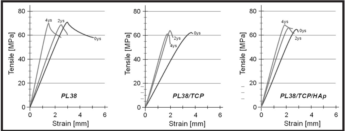
FIG. 3. Examples of tensile curves of dumbbell-shaped specimens. 0ys - initial samples; 2ys - tested after two years; 4ys - tested after four years.
