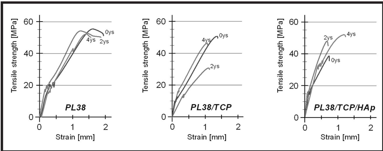
**FIG. 6. Example tensile curves of “N” type miniplates.**
