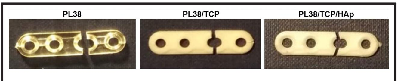
FIG. 10. Examples of miniplates after the mechanical testing. The characteristic manner of fracture can be seen.
