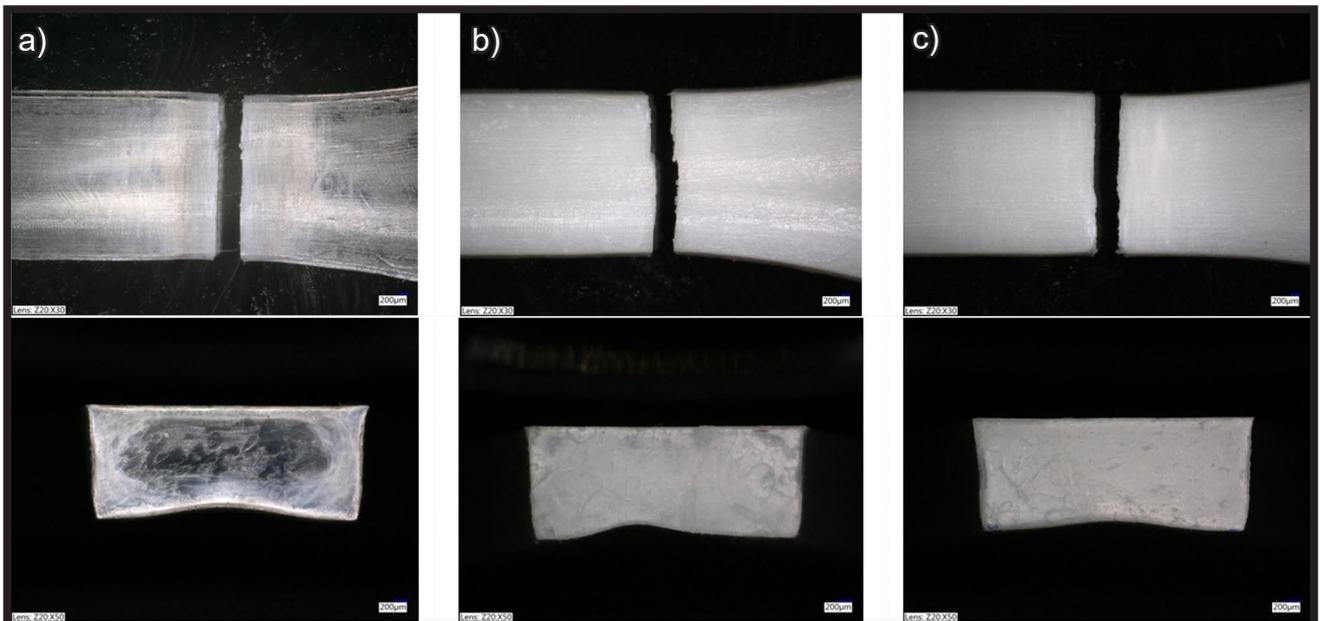
FIG. 4. Example of microscopic images of sample fracture (KEYENCE VHX-500, mag. x30; x50): a) PL38; b) PL38/TCP; c) PL38/TCP/HAp.
