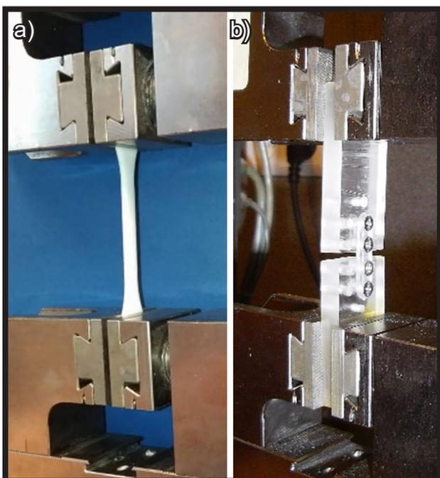
FIG. 2. a) Dumbbell-shaped specimen mounted and ready for testing; b) Simulated model of osteosynthesis with fixation miniplate.
