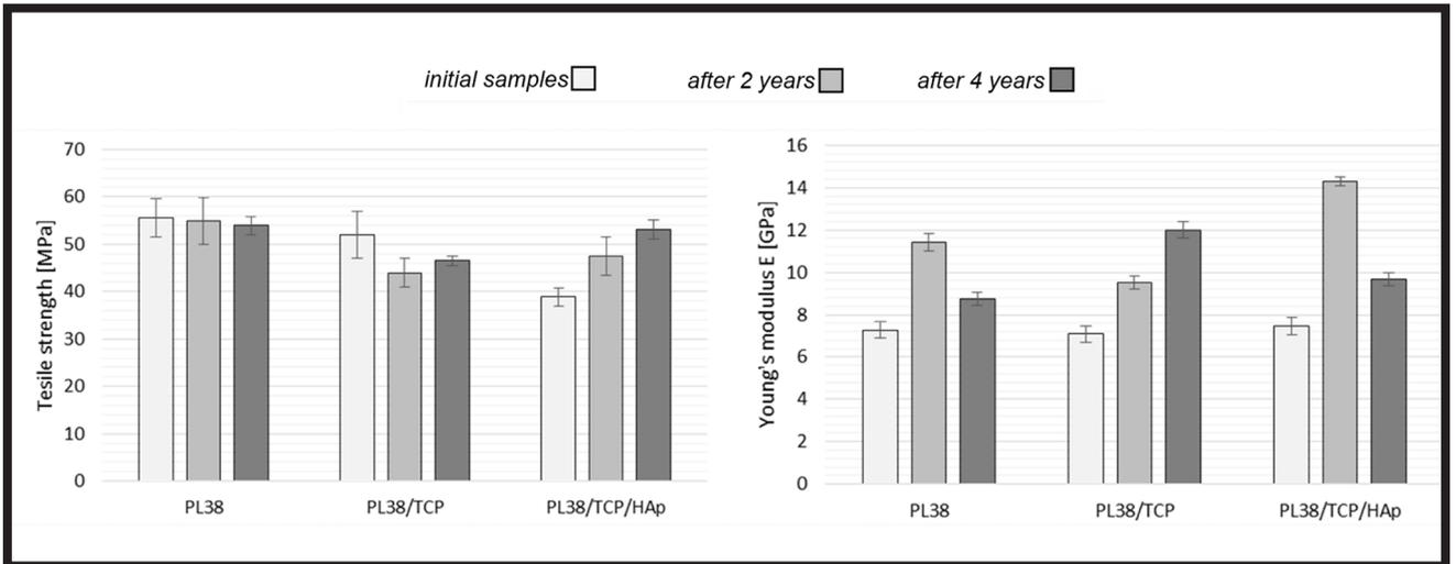
FIG. 8. Comparison of mechanical test results ( $R_m$  and  $E$ ) of the “N” type fixation miniplates of the initial samples, after 2 and after 4 years.
