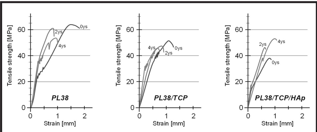
**FIG. 7. Example tensile curves of “R” type miniplates.**
