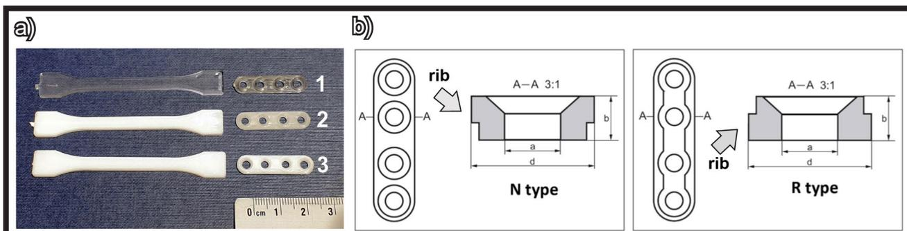
FIG. 1. a) Examples of dumbbell-shaped specimens and fixation miniplates used for testing. 1 - PL38; 2 - PL38/TCP; 3 - PL38/TCP/HAp; b) Schematic sketches of the I-shaped four-hole miniplate: type “N” with reinforcing rib from the bottom; type “R” with reinforcing rib from the top.
