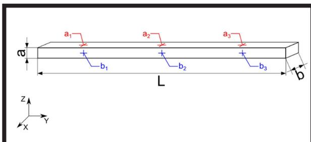
FIG. 2. Configuration of ultrasonic measurements of composite plate: L - along the length of plate, a - perpendicular to the thickness of plate, b - along the width of plate.
