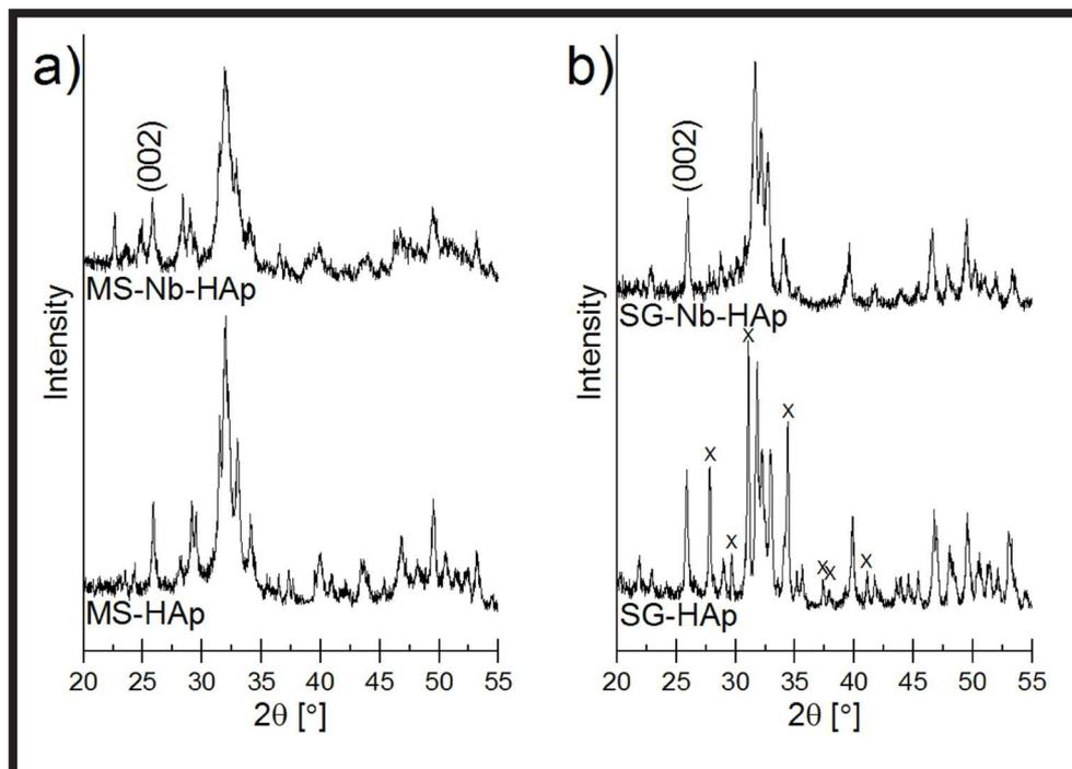
FIG. 3. XRD patterns of powders synthesized through: a) mechano-chemical synthesis, b) sol-gel method. X – the second phase with lower Ca/P molar ratio.
