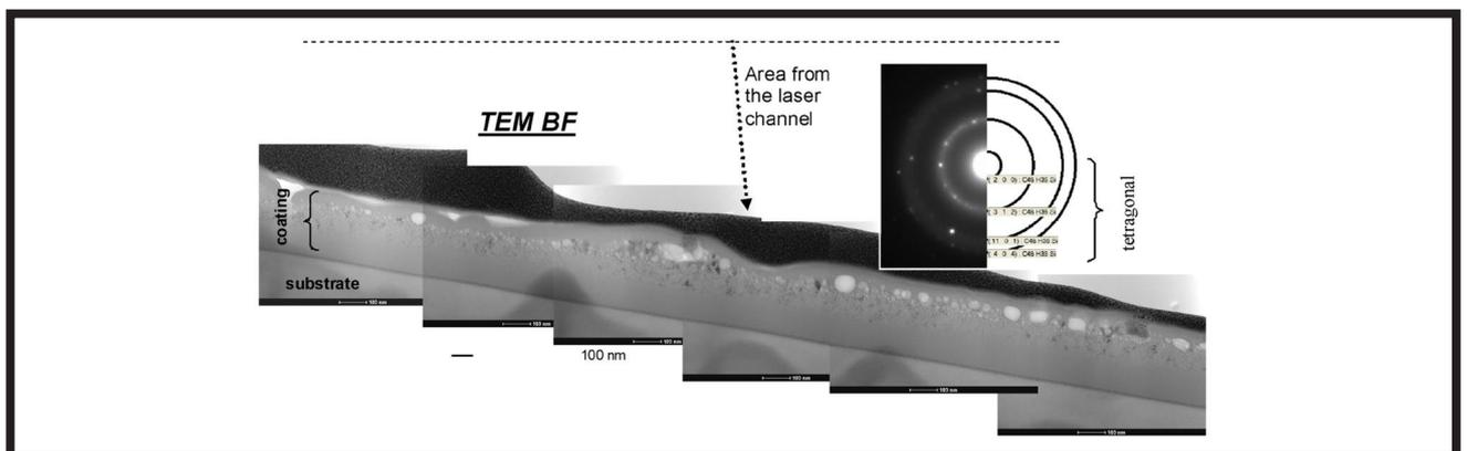
FIG. 6. The TEM microstructure in the tubule channel.
