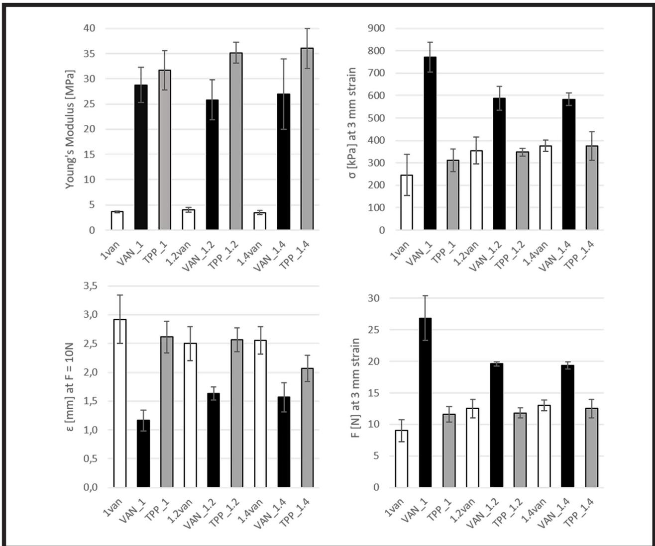
FIG. 8. The results after static compression test for the double crosslinked samples: Young's modulus, compression strength at 3 mm strain, stress at 3 mm strain, strain at stress  $F = 10 N$ ; triplets were tested for each type of material; error bars present standard deviations.
