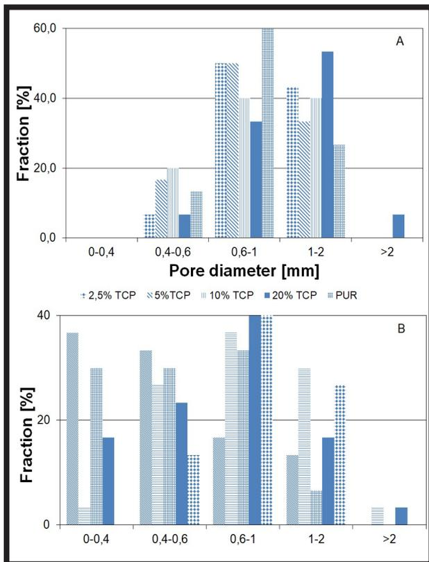
FIG. 4. Pore size distribution in composites with TCP (A) and HAp (B).
