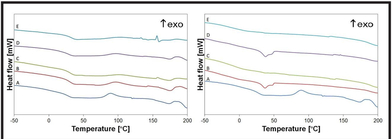
FIG. 2. DSC curves from the second heating for PU composites with HAp (left) and TCP (right): A) 20%, B) 10%, C) 5%, D) 2.5%, E) 0%.
