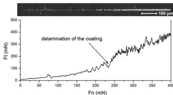
FIG. 2. Nanoscratch test curve.
