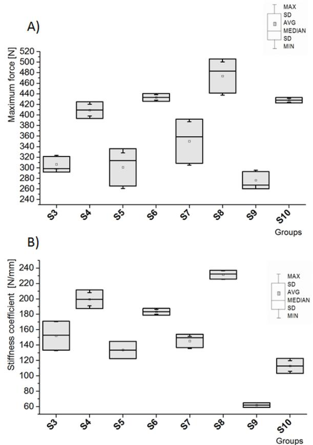
FIG. 1. The average value of a) the maximum force; b) the stiffness coefficient (k) of the tested groups of meshes.
