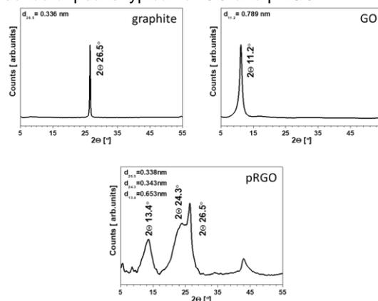
FIG. 1. Graphite, GO and pRGO XRD spectra.
