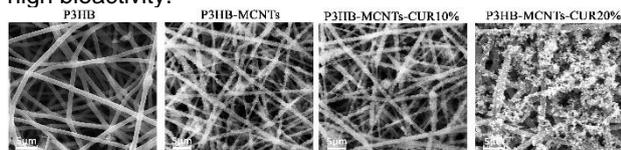
FIG. 1. SEM images after 4 weeks immersing in SBF.
