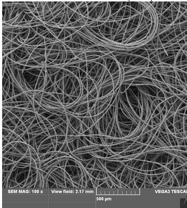
FIG. 1. SEM image of iron modified carbon nonwovens.
