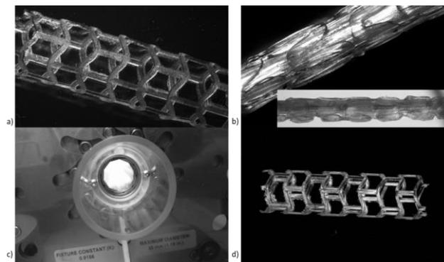
FIG. 1. Stent: a) before crimping process, b) crimped on balloon catheters, ready to implantation, c) crimper, d) opened after crimping (bright area-material tension)
