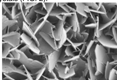
FIG. 2. Microstructure of bioactive layer on ZrO<sub>2</sub> scaffold.
