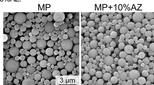
FIG. 1. SEM images of unloaded MPs (left) and MPs containing 10% AZ (right).
