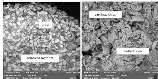
FIG. 1. The effects of machining of cartilage and bone in wet conditions: a) tool surface, b) chips after wet machining.
