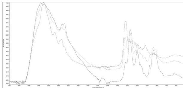
FIG. 1. IR spectra: collagen (dotted line), medium molecular weight chitosan (solid line), 50:50 mixture of chitosan and collagen (dashed line).
