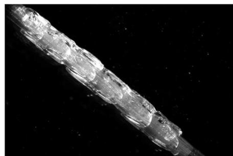
FIG. 4. Vascular stent clamped on the catheter.
