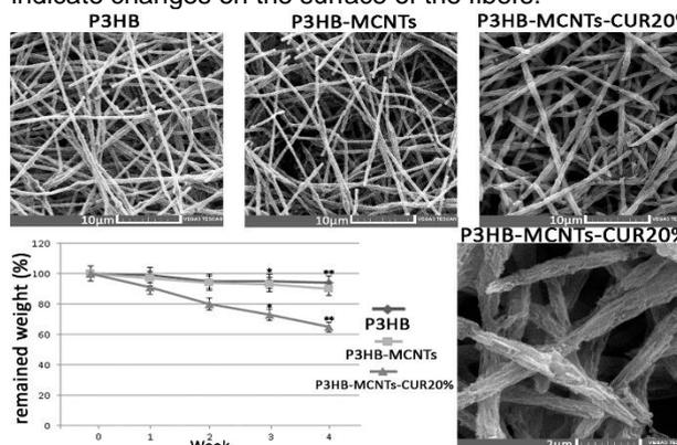
FIG. 3. SEM images and biodegradability rate in 4 weeks.
