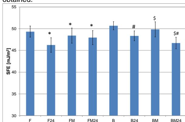
FIG. 1. SFE measurement results for materials immediately after polymerization and after 24 hours of incubation in distilled water. The symbols (\*) indicate statistically significant differences against material F, (#) - against material B, \$ - statistically significant difference between materials BM and BM24.
