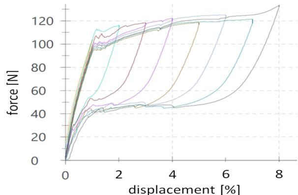
FIG. 2. Cyclic stress-strain wire curves measured for Ni-Ti wire.
