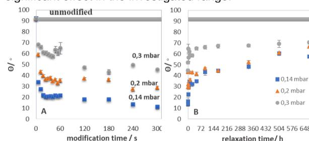
FIG. 1. Experimental water contact angles ( $\theta$ ) for different gas partial pressure (A), and the corresponding kinetic curves of plasma relaxation of activated polyurethane surfaces (B).
