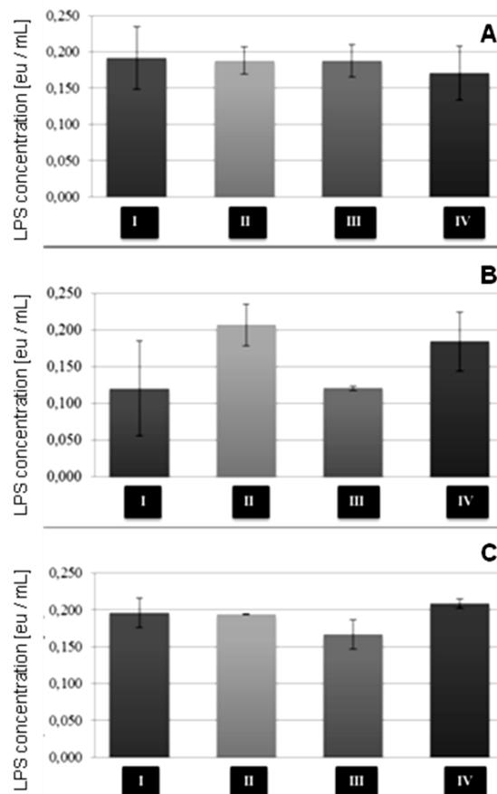
FIG. 1. Endotoxins (LPS) concentration in biofilms formed on the surface of the Ti6Al4V alloy samples by strains: A – DV/A, B – DV/B, C – DSM in various culture fluids: I – artificial saliva, II – artificial saliva simulating inflammation, III – Tyrode's fluid, IV – Ringer's solution.
