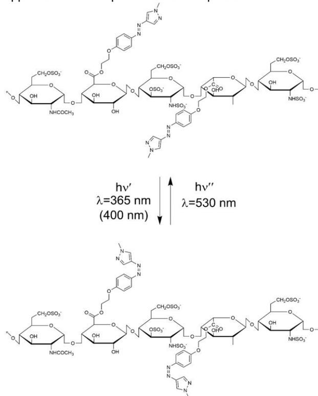
FIG. 1. Photoisomerizations in UFH heparin substituted with an AAP-type photoswitch.
