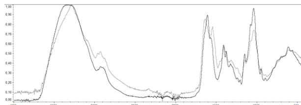
FIG. 1. IR spectra for 1.5% high molecular HA and 1.5% high HA with 0.25 g of albumin.
