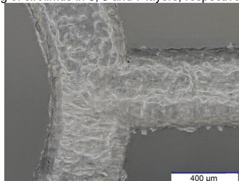
FIG. 1. Optical microscope image of the part of scaffold obtained from PLGA/oTMC coated with 7 layers of PLLA/TMC (1.0 %) and sirolimus using 60 kHz nozzle.
