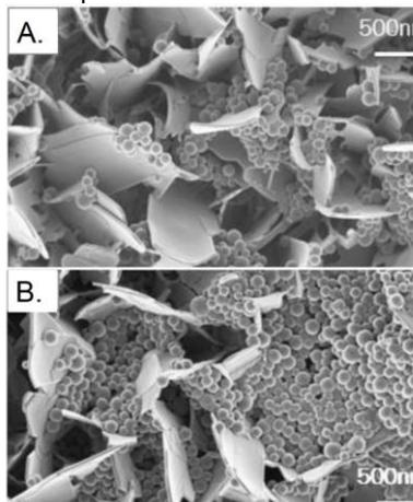
FIG. 3. SEM microphotographs of NPs deposited on ZrO<sub>2</sub> scaffolds during the CaP layer preparation process (A) and by drop-sitting method (B).
