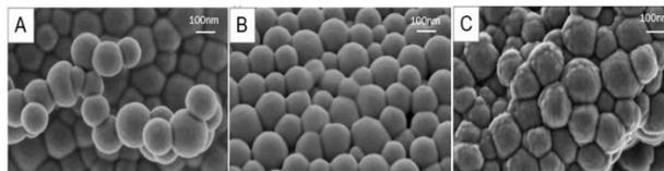
FIG. 1. NPs SEM characterization A. PLGA, B. PLGA-Gent, C. PLGA-Bct.
