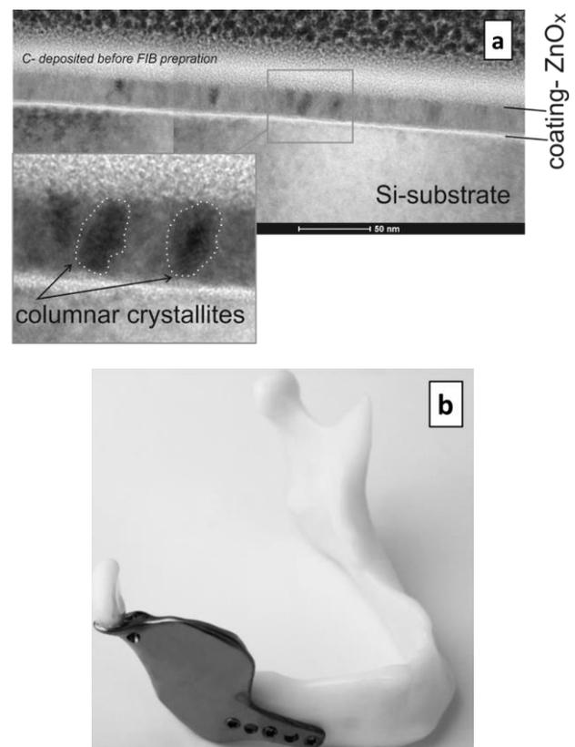
FIG. 1. (a) Transmission electron microscopy image of the ZnO coated surface. (b) Final prototype of the composite implant.
