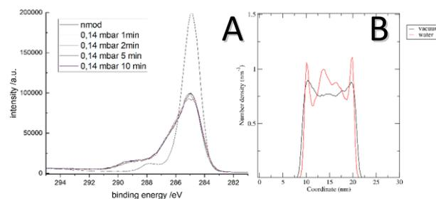
FIG. 1. Representative C1s XPS spectra of unmodified (nmod) and oxygen plasma modified polyurethane (A) accompanied by a representative image of polyurethane chains N atom distribution in the MD simulation box (B).
