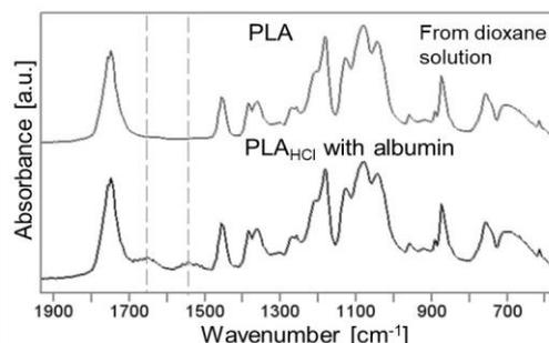
FIG. 1. ATR spectra of selected PLA samples.
