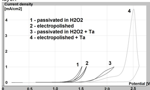
FIG. 1. The corrosion resistance of NiTi uncoated and coated by Ta<sub>2</sub>O<sub>5</sub> layer.
