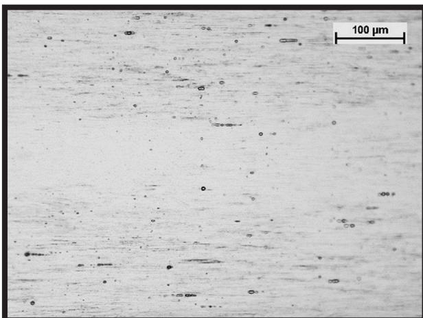
FIG. 3. The microstructure of the G&H Orthodontics orthodontic wire. Visible fibrous texture and precipitations of the  $Cr_{23}C_6$  carbide arranged in bands. Etched state. LM
